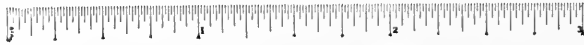
FIG. 20—Photographic Enlargement Measure, graduated in 64ths of an inch, to be photographed with the object to serve as a permanent record of the degree of enlargement.
